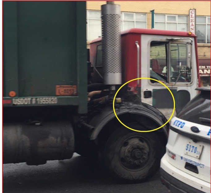
The fender of this Brooklyn private waste truck is held together by duct tape.
